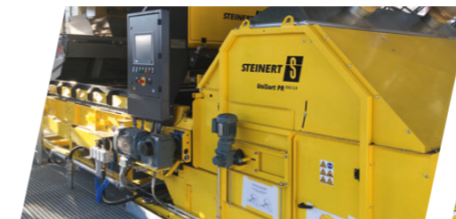
Sorting wood products using UniSort PR EVO 5.0
