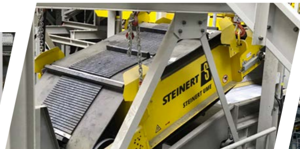
Separating ferrous metals using STEINERT UME
