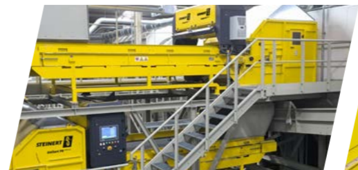
Sorting plastics and wood using UniSort PR EVO 5.0
