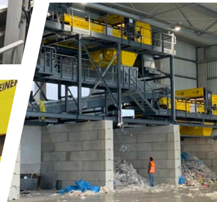
Sorting paper & cardboard as well as films using UniSort Film EVO 5.0
