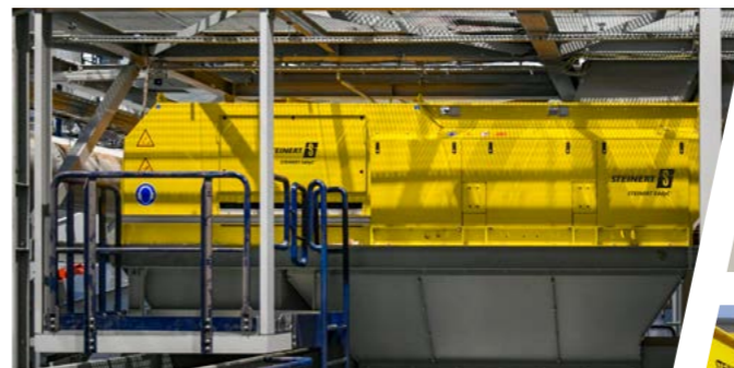
Recovery of non-ferrous metals using STEINERT EddyC
