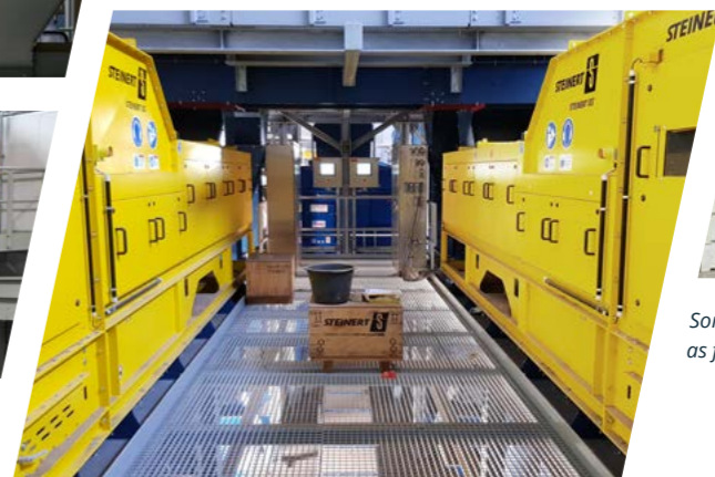
Sorting metals and stainless steel using STEINERT ISS
