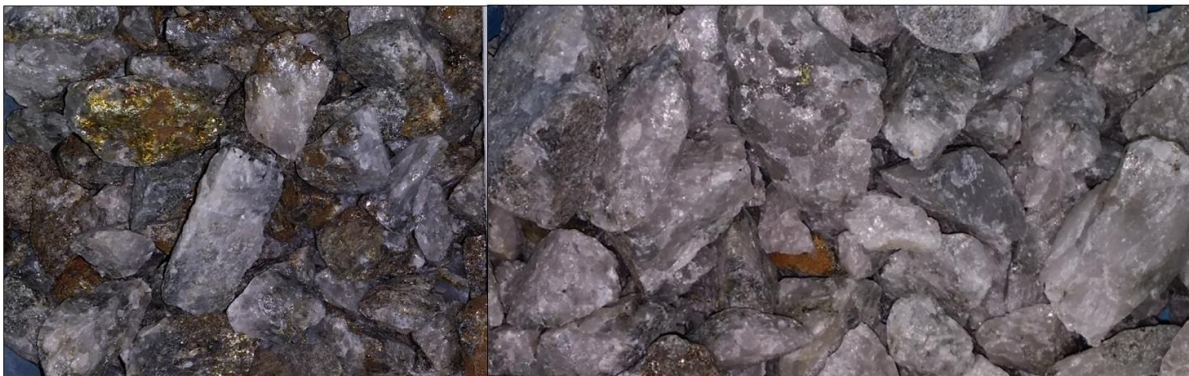
Figure 6 - Gold-bearing ore samples: Sulphides (left), Quartzite (right).
