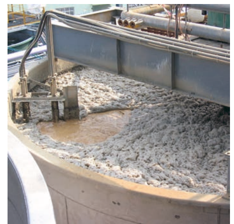
The BIOX process was developed for the pre-treatment of refractory concentrates ahead of conventional cyanide leaching for gold recovery
