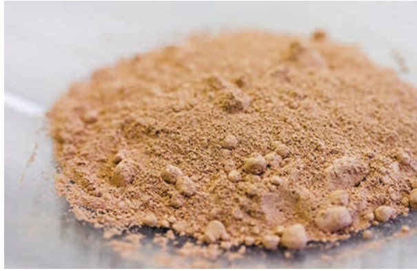
Finely ground gold ore for biological processing with Green Mining technologies developed by BRAIN and CyPlus
