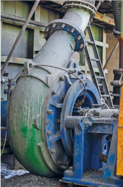
Kanowna Belle Warman pump - Weir Minerals has celebrated 80 years of innovation with the Warman slurry pump, which remains one of the most popular high wear slurry pumps on the market
