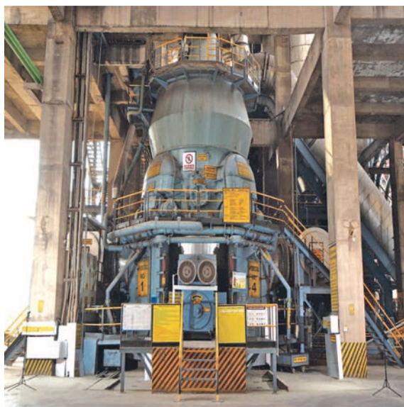
Currently the largest Loesche mills have drive-power capabilities up to 10 MW. The mills have redundant systems to avoid machine failures and to ensure high levels of availability. They operate dry and require substantially less power than SAG Mills for comparable grinding capacities of up to 2,000 t/h
