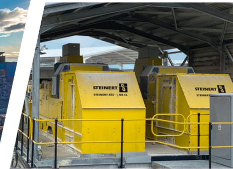
STEINERT KSS | NR CL pre-concentrates white dolomite
