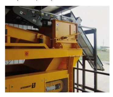
Efficient non-ferrous extraction using an eccentric pole system Proven in operation for 25 years with more than 3,500 units sold, the eccentric pole system in the STEINERT non-ferrous separator prevents damaging iron particles from adhering and concentrates power where it is needed. The system's adjustability increases the yield by another 50%. Altogether the best possible conditions for obtaining a ready-to-sell non-ferrous product in the famous STEINERT quality.
