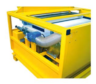
Working widths of up to 1500 mm, belt thickness down to 150 micron for a maximum field strength and knife splitter for precise separation.
