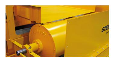
The field is constant the entire width, but alternates in the drum's direction of travel, recommended for a clean magnetic product. Benefits: The first axial pole is stronger than the others to draw up the ferrous items, then the other poles flip and clean the material. This means the knuckles are not missed and the drum edges are fully utilized. Better than traditional side plate mounted bearings, STEINERT uses larger shafts and drum bearings with independent housings.
